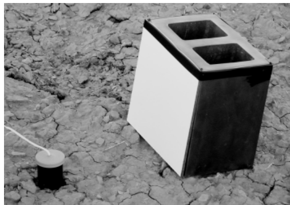
FIG. 3—Setup for background discrimination demonstration, showing a 35-mm film can of fireworks flash powder and a collection surface attached to a heavy metal support.
